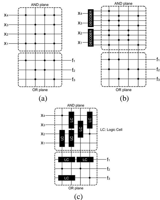
Figure 1. Structures of (a) the conventional PLAs (b) with input decoders and (c) the proposed PLA.
