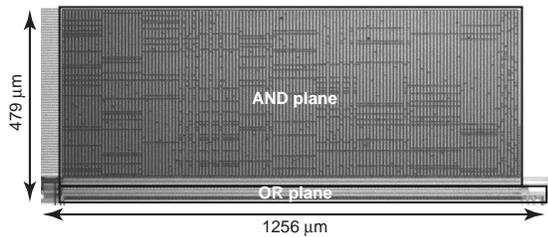
Figure 7. Chip microphotograph.
