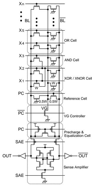
Figure 2. Basic circuit of the proposed PLA.
