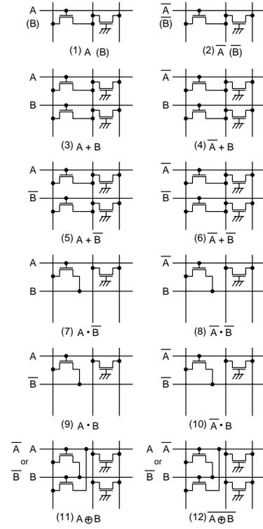
Figure 3. Logic cells (LCs) for the basic circuit.
