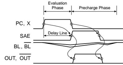
Figure 4. Timing diagram of the control signals.
