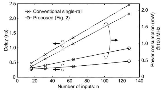
Figure 6. Basic circuit comparison for delay and power consumption (0.35- $\mu\text{m}$  CMOS technology, 3.3-V  $V_{DD}$ ).
