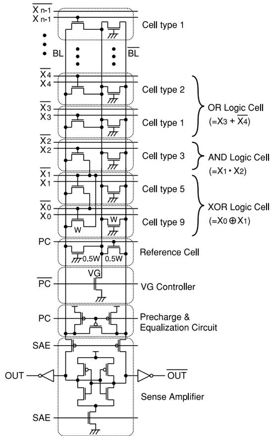
Fig. 2 Basic circuit of LCPLA.
