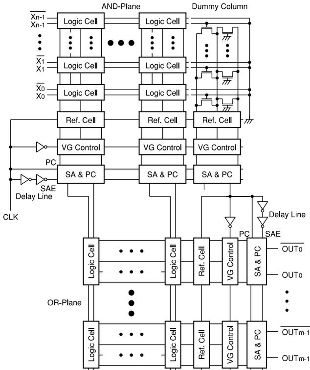
Fig. 6 Overall configuration of LCPLA.
