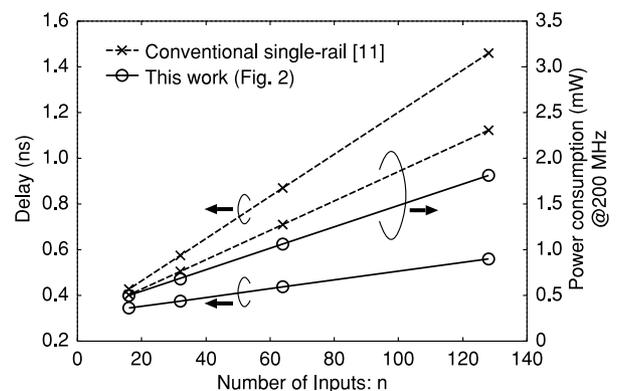
**Fig. 7** Basic circuit comparison in terms of delay and power consumption (0.35- $\mu\text{m}$  CMOS technology, 3.3-V power supply).
