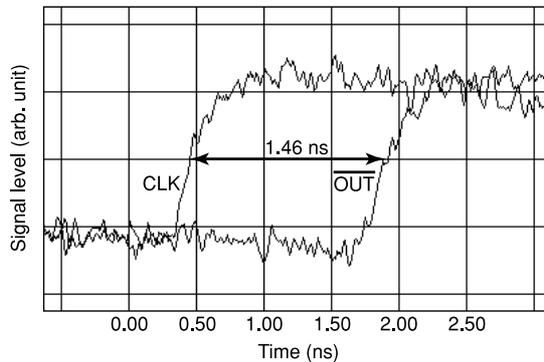
Fig. 10 Measured waveforms by an electron-beam tester.
