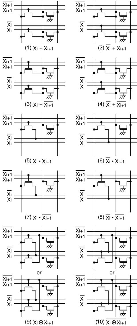
Fig. 4 2-input logic cells (LCs) using the basic logic cells.
