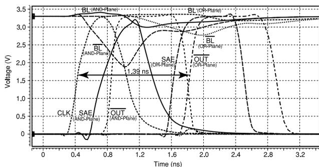
**Fig. 8** Simulated waveforms of the LCPLA.
