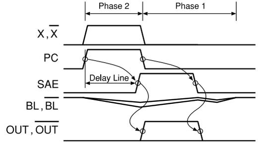
Fig. 5 Timing diagram of control signals, input and output signals, and bit-line potentials in a basic circuit.
