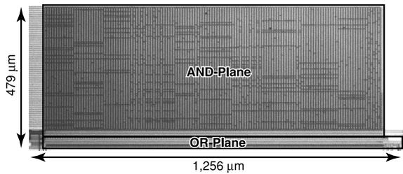
Fig. 9 Chip microphotograph of the LCPLA.
